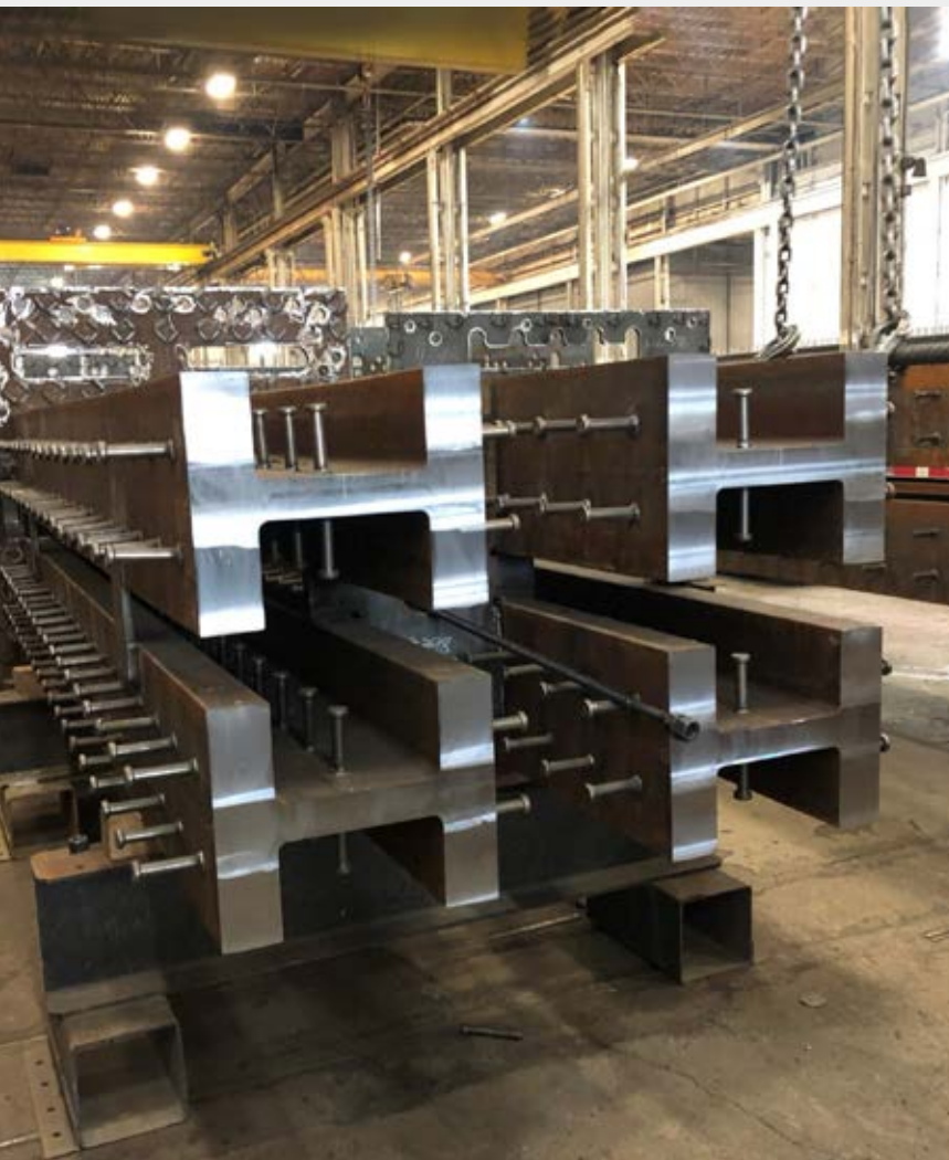
Fig. 7: Composite Mega Column in the fabrication shop
