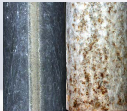
Magnelis® ZM310 welded and re-protected Post-galvanised welded
