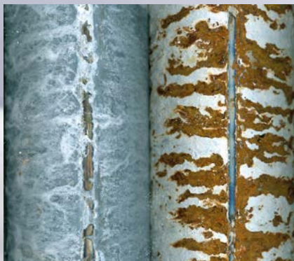
Magnelis® ZM120 welded, not re-protected Galvanised Z275 welded, not re-protected
